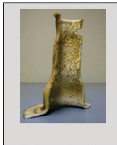
Typical permeation failure of isostatically formed liner
