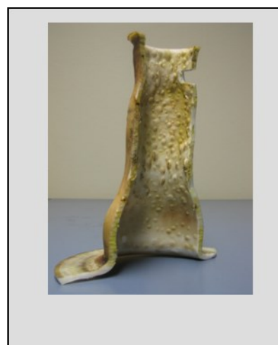
Typical permeation failure of isostatically formed liner
