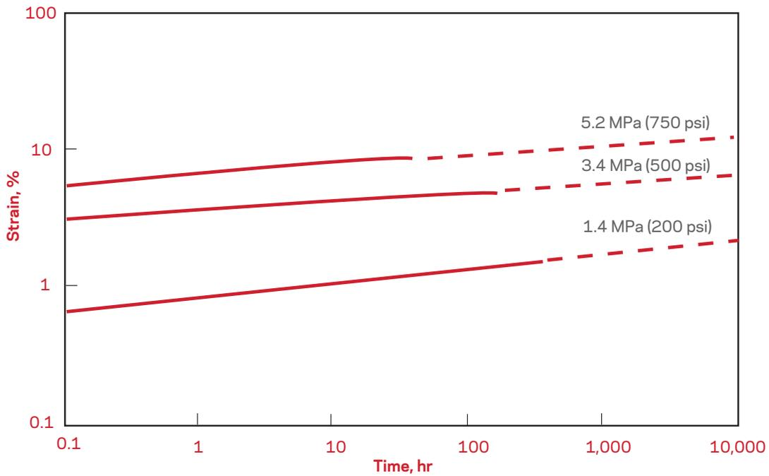
Figure 9a. Total Deformation versus. Time Under Torsional Load at 23 °C (73 °F)
