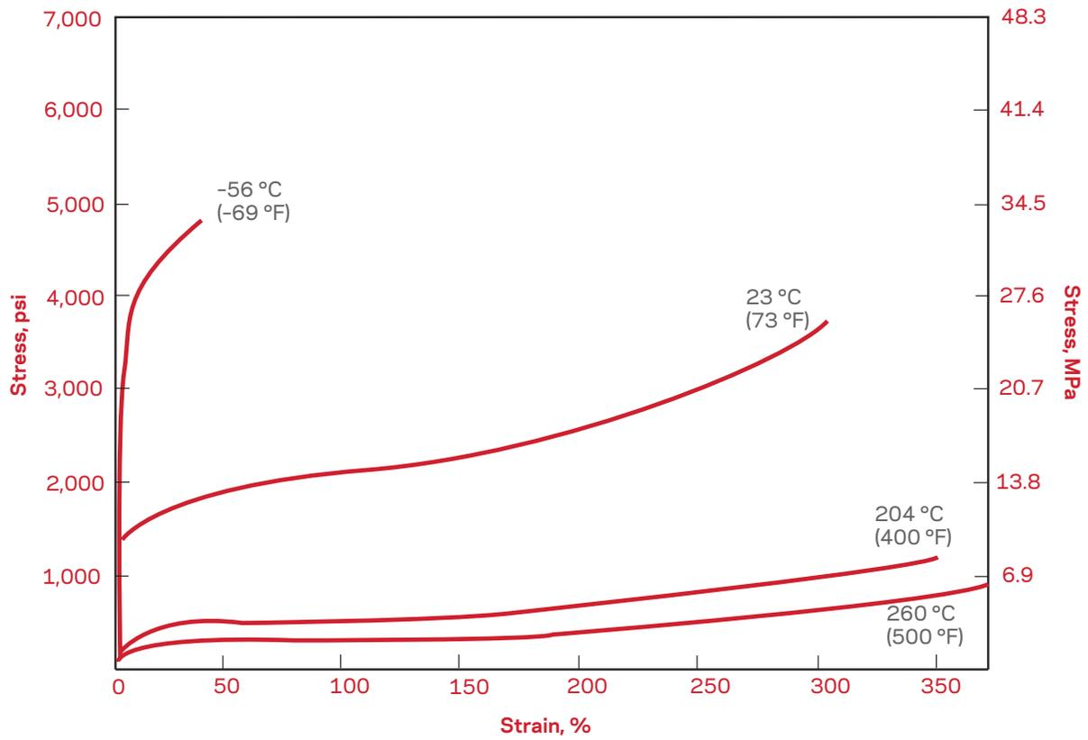
Figure 3. Tensile Stress versus Temperature at Constant Strain
