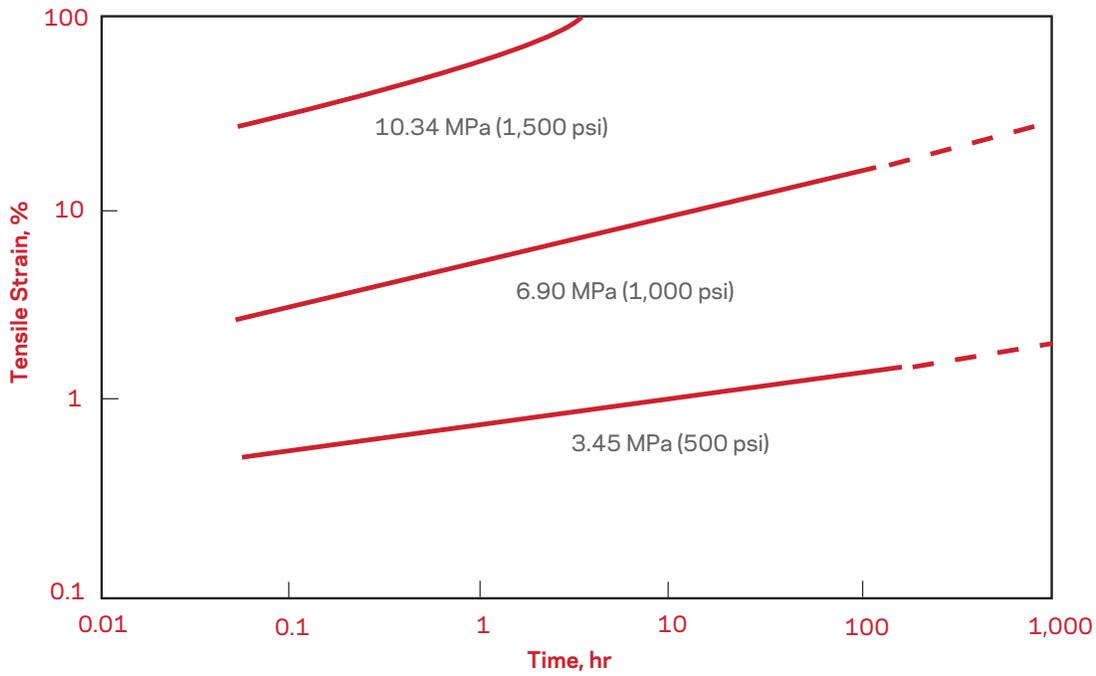
Figure 7c. Total Deformation versus Time Under Tensile Load at 100 °C (212 °F)
