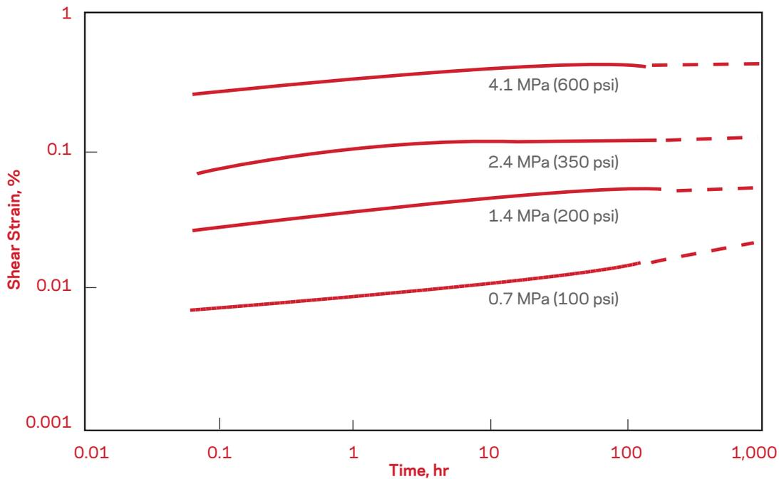
Figure 10a. Tensile Strength Relaxation at 23 °C (73 °F)
