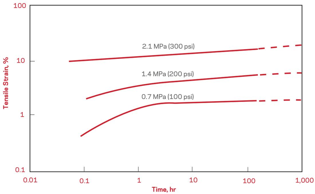
Figure 8a. Total Deformation versus Time Under Compressive Load at 23 °C (73 °F)
