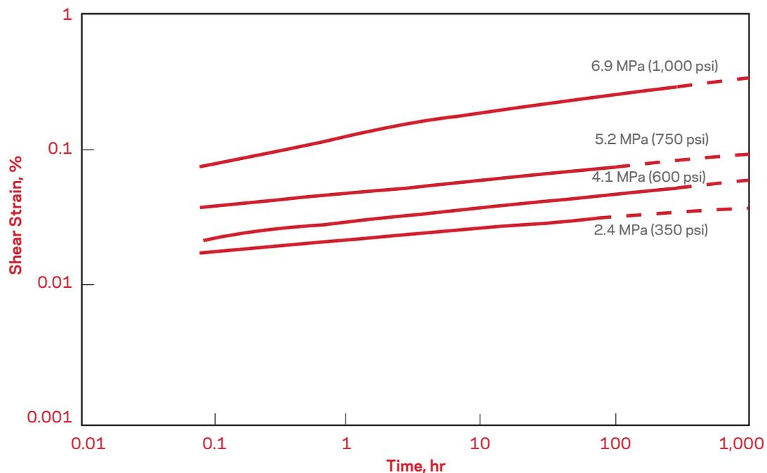
Figure 9b. Total Deformation versus Time Under Torsional Load at 100 °C (212 °F)
