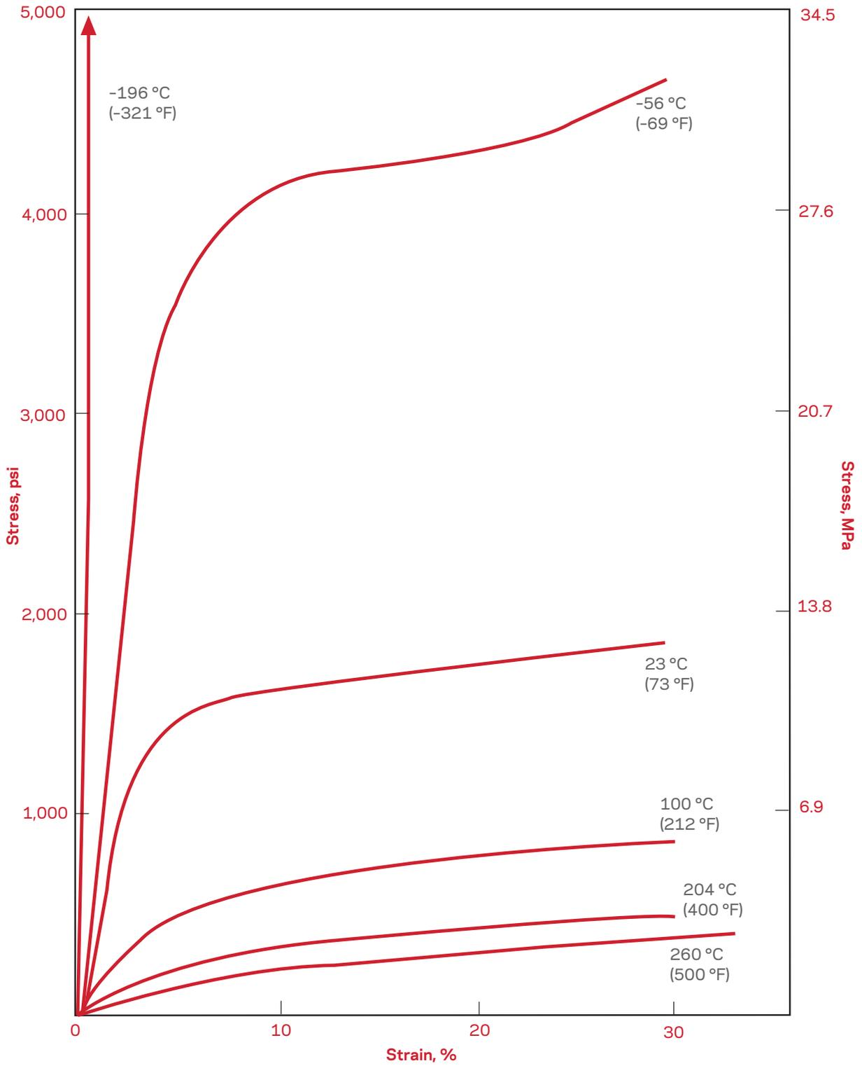
Figure 2b. Stress versus Strain in Tension
