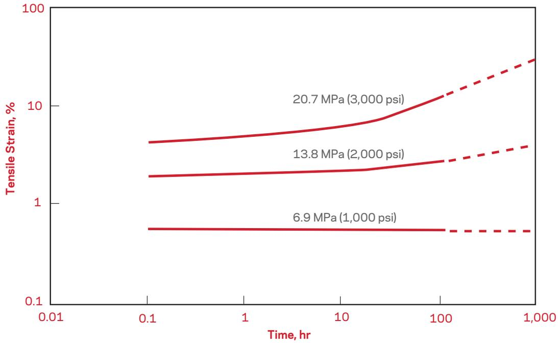
Figure 7b. Total Deformation versus Time Under Load at 23 °C (73 °F)
