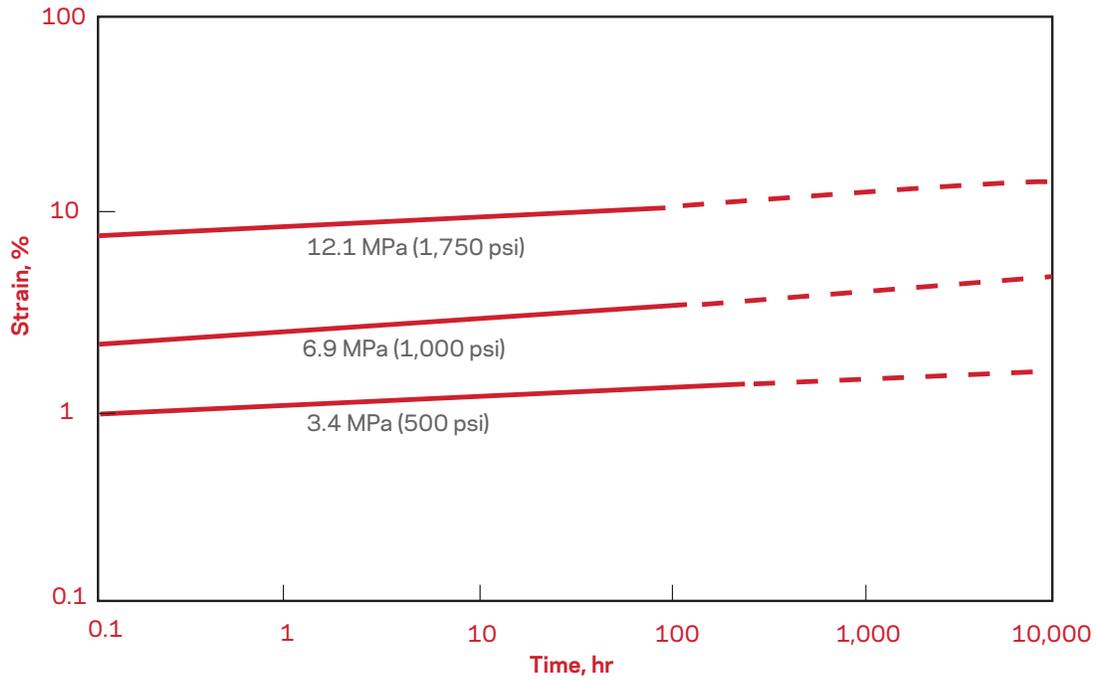
Figure 8b. Total Deformation versus Time Under Compressive Load at 100 °C (212 °F)
