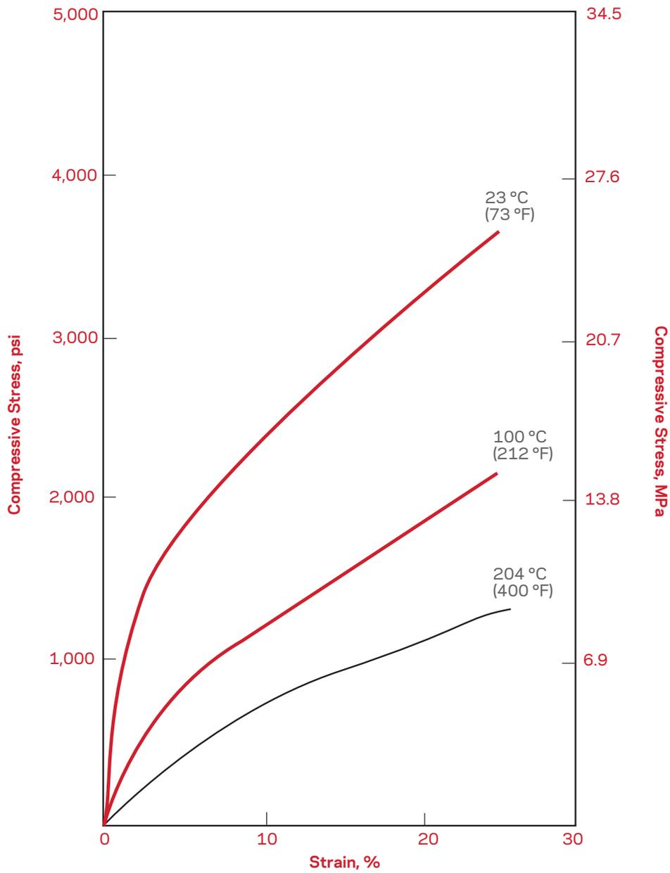
Figure 5. Stress versus Strain in Tension and Compression (ASTM D695)
