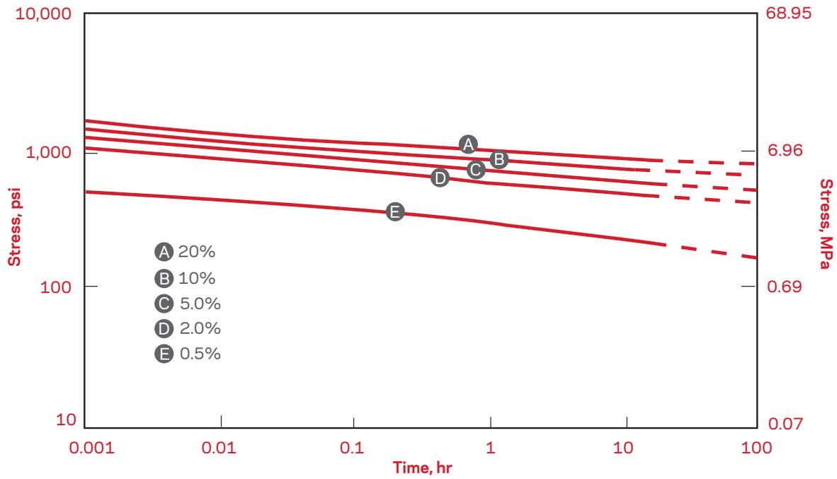
Figure 10b. Tensile Strength Relaxation at 100 °C (212 °F)
