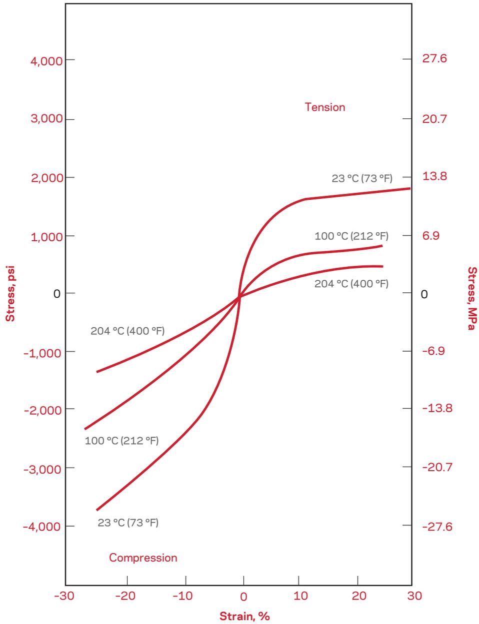
**Figure 6. Stress versus Strain in Shear to 20%**
