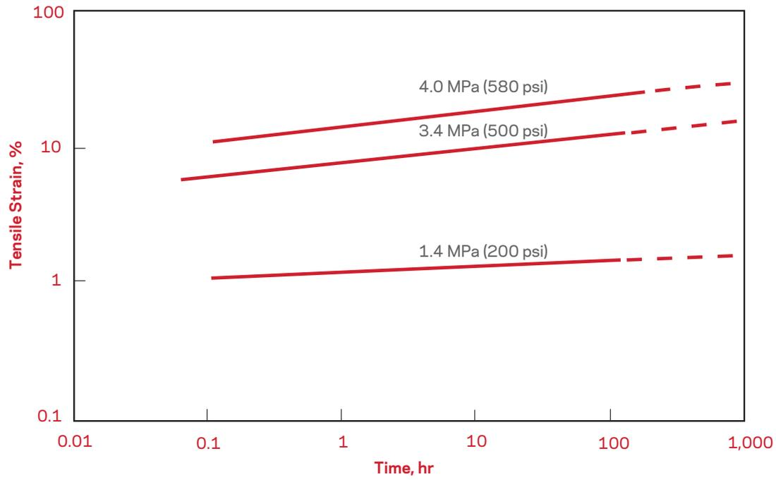
Figure 7d. Total Deformation versus Time Under Tensile Load at 200 °C (392 °F)
