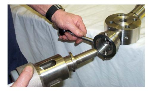
With your free hand rotate the operating lever mounted on the valve connection clock wise by 90 degrees. The syringe has a cam attachment, you will be able to feel the cam mechanism engaging and locking in position. As the cam engages the sample device automatically opens
