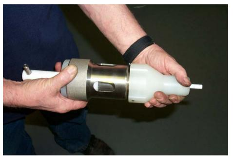
CRP Ltd Todmorden Road, Littleborough, Lancashire, OL15 9EG. Tel. +44(0)1706 756400. Fax. +44(0)1706 379567 web: www.crp.co.uk e-mail: <u>enquiry@crp.co.uk</u> The sample can be taken from the syringe by pushing the plunger closed, the sample is dispensed through the tube at the end of the carrying cap
