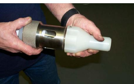
Offer the syringe unit carefully up into the sampling connection in the sampling device.
