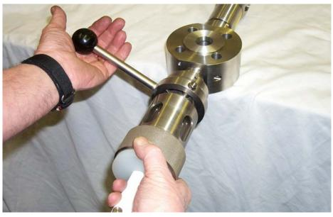
Fit the carrying cap again to the syringe sampler. The sampler can then be safely transported to the laboratory for example.
