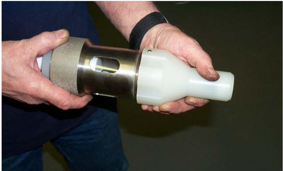
Offer the syringe unit carefully up into the sampling connection in the sampling device.
