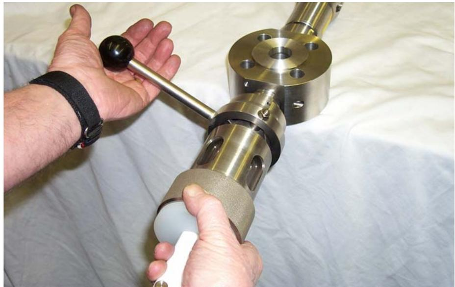
Fit the carrying cap again to the syringe sampler. The sampler can then be safely transported to the laboratory for example.
