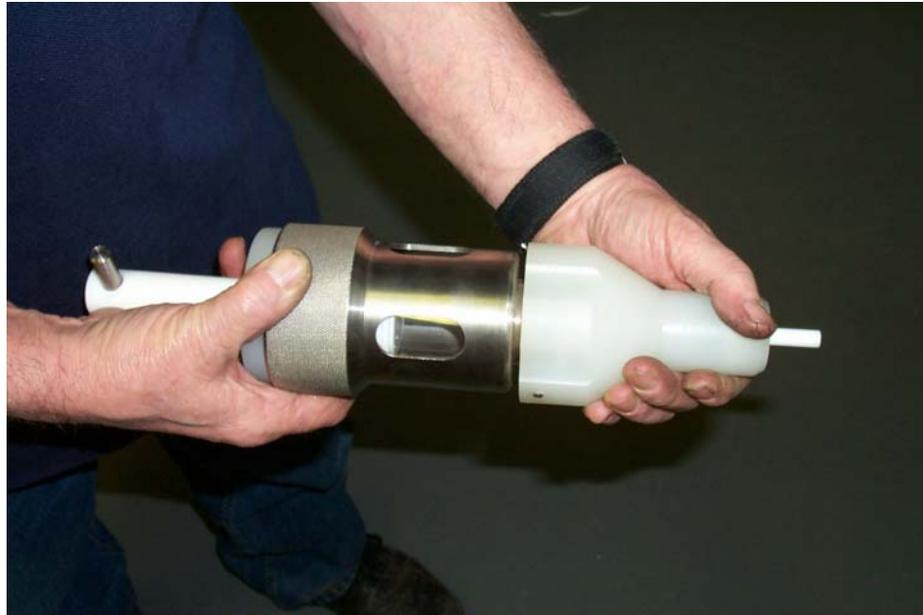
The sample can be taken from the syringe by pushing the plunger closed, the sample is dispensed through the tube at the end of the carrying cap
