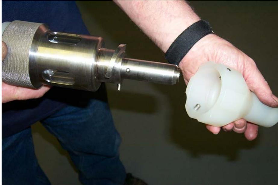
To dispense the sample from the syringe sampler, remove the carrying cap and fit the dispensing cap. This is done by rotating the cap on the cam mechanism until it locks.
