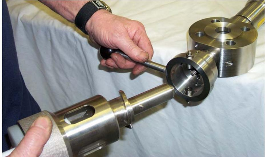
With your free hand rotate the operating lever mounted on the valve connection clock wise by 90 degrees. The syringe has a cam attachment, you will be able to feel the cam mechanism engaging and locking in position. As the cam engages the sample device automatically opens the valve in the sampling body, a representative sample flows from the pipeline into the borosilicate glass cylinder under pressure from the pipeline.
