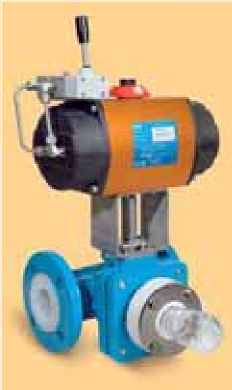
Safety pneumatic automation for AtoPro™ sampling ball valves, consisting of a Norbro 180° spring return actuator type 25RB33. Manual operated by a Hoebriger automatic safety device with dead man function.
